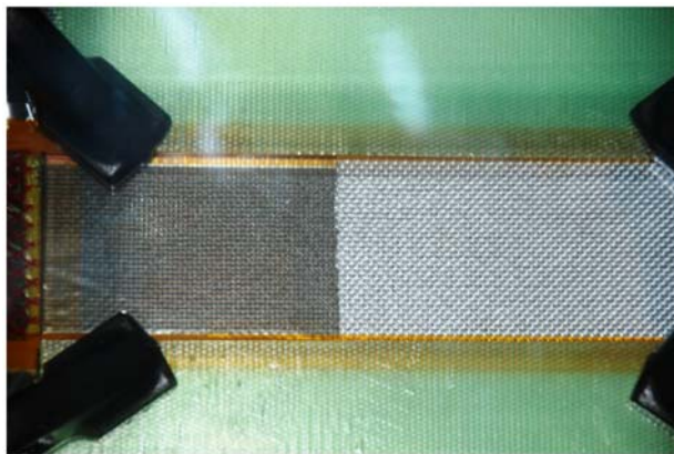
Figure 2. Image of flow front during one-dimensional RTM.
